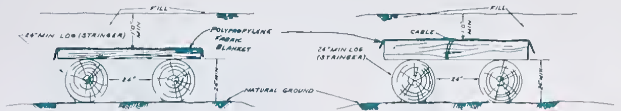
ALTERNATE CABLE LASHED LOG CULVERT
